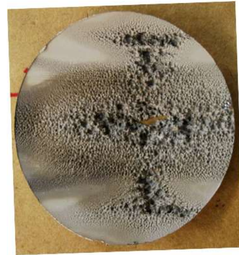
Target 1, center disk Bulk flow side After cleaning
