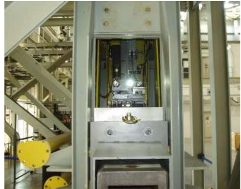
CVI Robot Lowered to the Base of the mockup test stand
