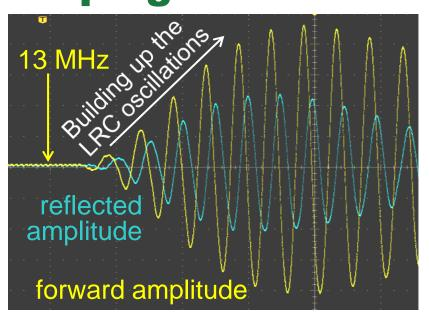
•RF build-up was studied with 4-week-old source #2 using a 2 MHz directional coupler on ground.
