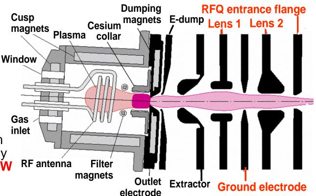
The two-lens, electro-static LEBT is 12-cm long. Lens-2 is split into four quadrants to steer, chop, and blank the beam.
