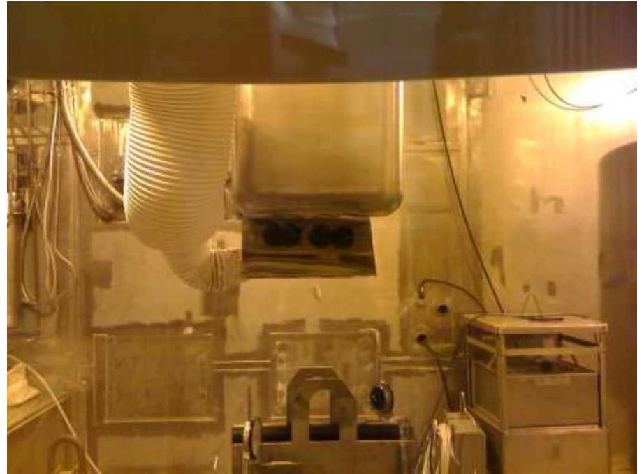
View of Target nose following the fourth cutting operation
