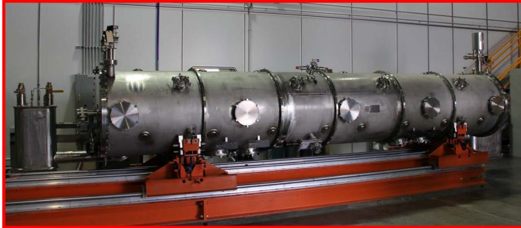
High beta spare has been in service since the summer of 2012 and all four cavities reached 16 MV/m, STS specification
