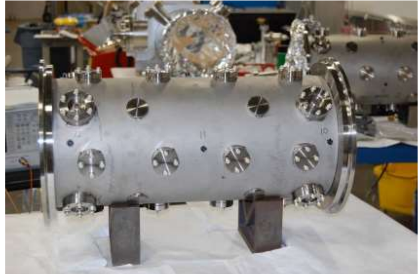
Damper Vacuum Vessel
