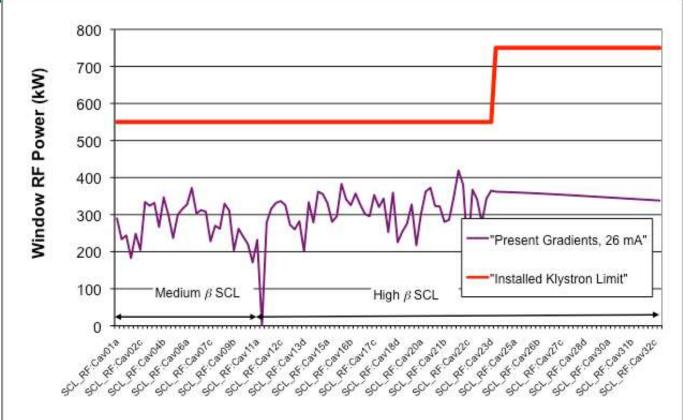
Using the PUP cavity gradients, the present RF equipment is sufficient for 26 mA
