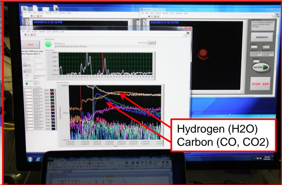
Hydrocarbon oxidation by-products from HB59 cavity
