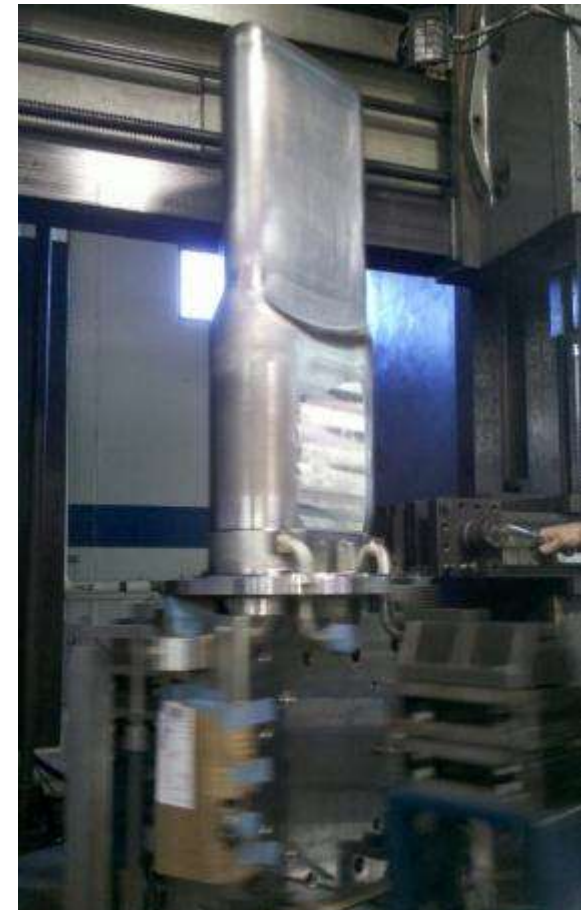
Final machining of ORTE-001 for mounting the inflatable seal
