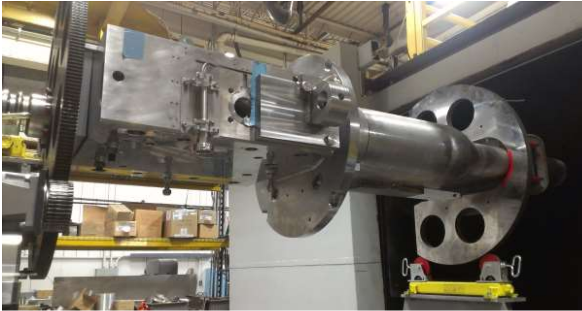
ORTE-001 Target Module mounted on e-beam weld tooling just prior to final weld pass
