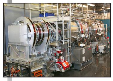
an unprecedented dynamical range of six decades from 1 ps  $< \tau < 350$  ns. The design of the spectrometer takes advantage of recent progress in neutron optics and polarizing supermirror microbenders, resulting in considerable gains in polarized neutron flux over a wide wavelength range. Performance is also extended by a position-sensitive, twodimensional detector with a broad detection region. As a result, the effective data rate will gain an additional factor of 5 in addition
