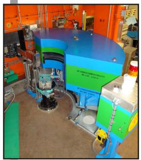
depending on which reflection is in the diffracting condition: (113) 2.41 Å, (115) 1.54 Å, and (117) 1.12 Å. The takeoff angle from the monochromator is fixed at 90°, and the minimum peak full width at half maximum (FWHM) is 0.2°. There are two choices of premonochromator collimation (α, = 12' or open) and three choices of presample collimation ( $\alpha_2 = 16, 21, \text{ or } 31$ ') that allow the operation of the instrument in highresolution or high-intensity modes.
