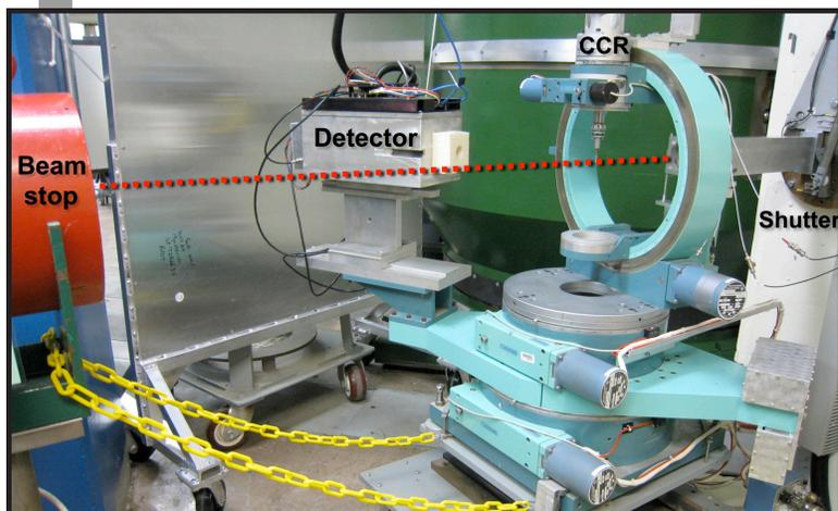
reflection from planes of the  $\langle 011 \rangle$  zone ensures sharp diffraction peaks in specified ranges of detector angles by control of the horizontal radius of curvature. Any plane from the  $\langle 011 \rangle$  zone can be set in Bragg position, but only the (331), (220) with (440), and (111) with (333) reflections are of practical interest. For the fixed monochromator angle of  $48^\circ$ , these reflections provide principal incident
