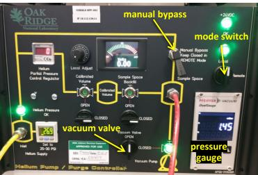
Figure 3. Helium Pump / Purge Controller
