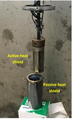
Figure 5. Sample stick and heat shields.
