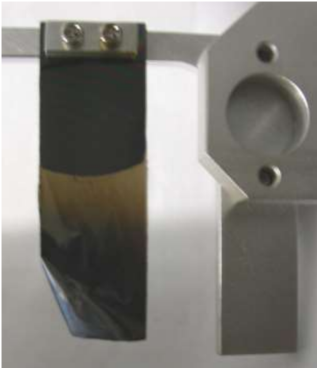
Foil #601, from position #6, removed 29/Oct/07. Curl is toward upstream.
