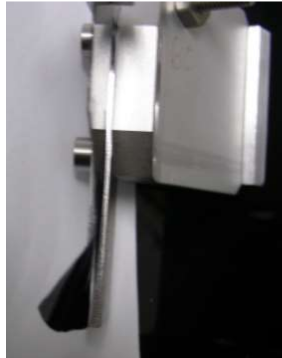
Foil #601, from position #6, removed 29/Oct/07. Curl is toward upstream.
