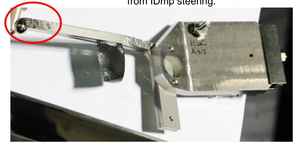
HBC A-4.7. End melted when adjacent foil raised for IDmp steering studies? Or RCE from adjacent foil? ~13.5 hours at 1.2 MW.
