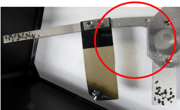
#1839, used for 1.1 – 1.2 MW for a few weeks, then 1.4 MW demonstration for a few minutes, and then 1.3 MW for ~32 hours.
