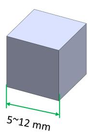
For strong neutron absorbing samples (e.g. containing a large fraction of B, Gd, etc), small TexBall samples are recommended.
