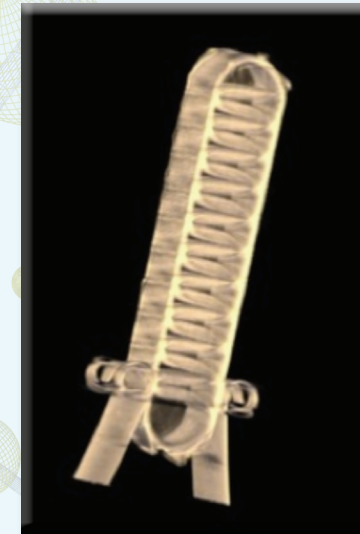
Neutron CT of EGR cooler measured at the High Flux Isotope Reactor prototype beam line.
