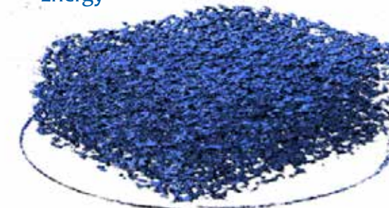
Computed Tomography of Li distribution ( Li_2O_2 ) in a control battery.
