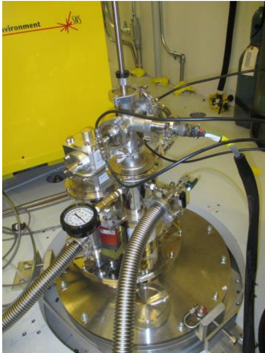
JANIS closed-cycle refrigerator (5-600K)
