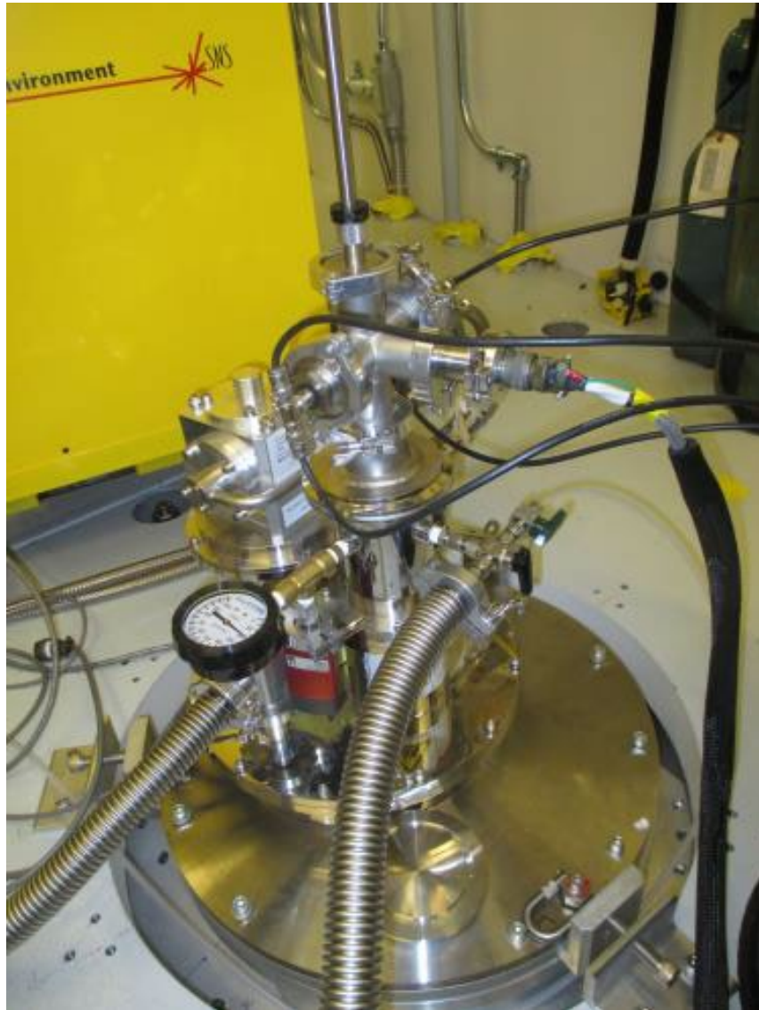
JANIS closed-cycle refrigerator (5-600K)
