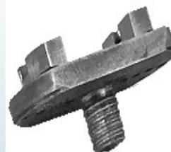
"Thread" sample holder onto Displex cold finger. Make sure that absorbing ring is properly fitted while threading.
