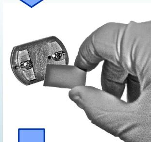
Place sample on surface and secure with clips
