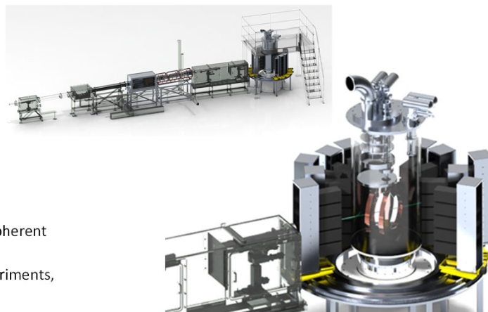
DNP-IMAGINE-X: conceptual design of the new DNP sample environment, detector banks and upstream neutron polarization and spin-flipper system, installed at the end station of the current IMAGINE beamline
