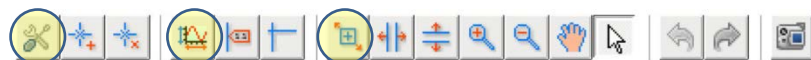
Figure 6. Graph Toolbar, with the Configure Settings, Perform Autoscale and Rubberband Zoom buttons highlighted (left to right).
