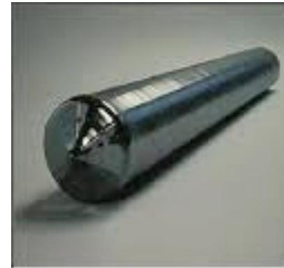
Silicon is used for monochromator crystals as it can be easily obtained and has good thermo-mechanical properties for cooling.
