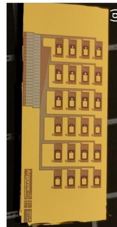
The TES is biased on the superconducting transition to maximize  $\alpha$ , a measure of the sensitivity of the device.
