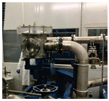
Figure 8.28. Prototypical GLS installed at TTF.
