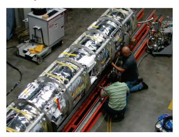
Figure 3.12. Cryomodule cold mass assembly.
