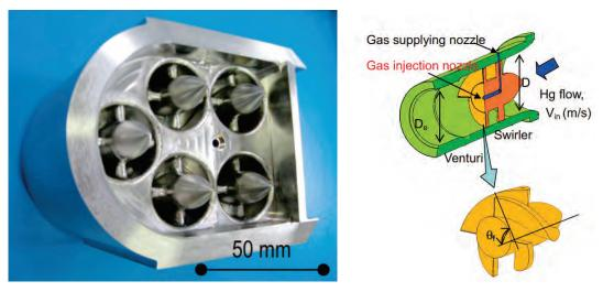
Figure 8.8 Picture of the swirl bubblers assembly used at J-PARC (left) and schematic of the cross-section of a single swirl bubbler (right).
