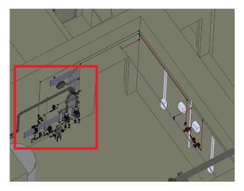
Figure 6.37. Target wall compressors.
