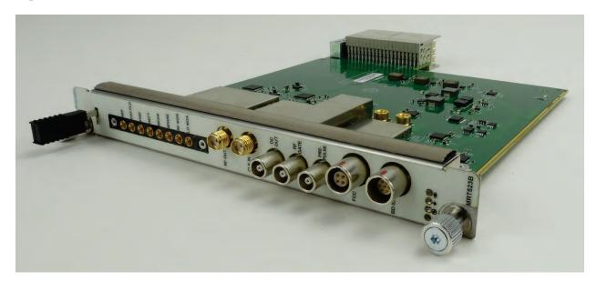
Figure 4.11. Field control module-II rear transition module.
