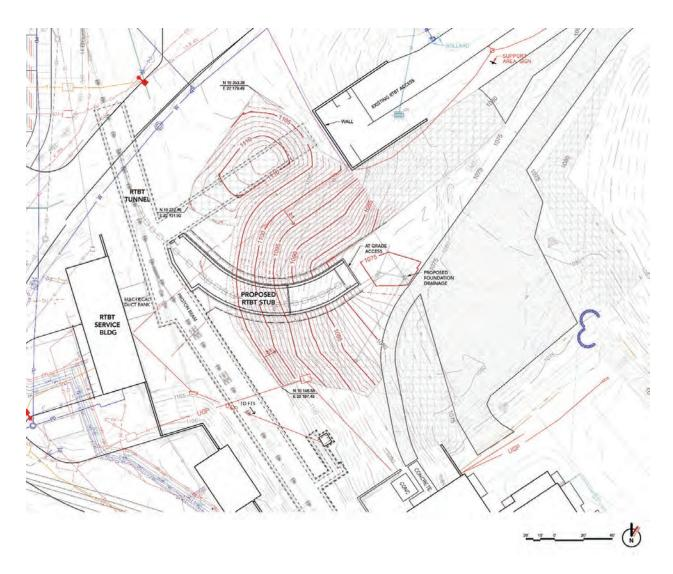
Figure 7.7. Backfill plan and new site drainage.
