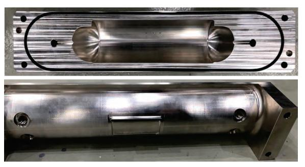
Figure 8.2. Stainless steel nose for the visual target for the heat transfer experiments.
