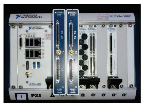
Figure 4.37. The new National Instruments NI 5751 FPGA modules replace the obsolete module and offer additional I/O and enhanced functionality.
