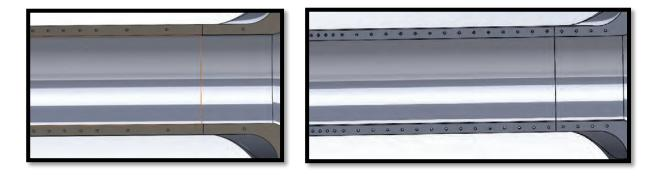
Figure 6.48. (L) Current water-cooled shroud cooling channels; (R) PPU water-cooled shroud target channels.
