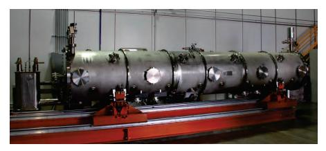
Figure 3.10. SNS spare high-beta cryomodule.
