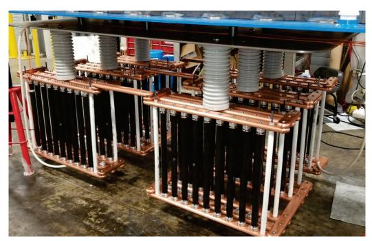
Figure 4.22. Dummy high-voltage resistive load for modulator testing, shown removed from the oil tank. Changing individual resistive elements permits customizing the load resistance to mimic a variety of klystron load impedances.
