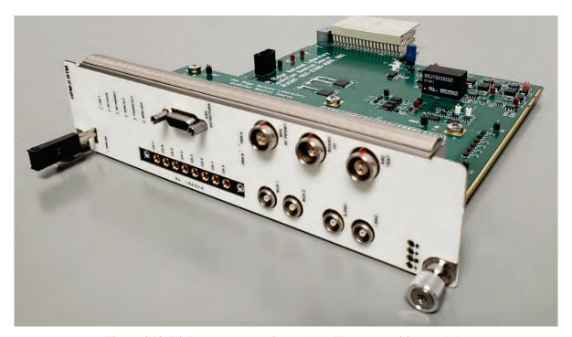
Figure 4.12. High-power protection module-II rear transition module.
