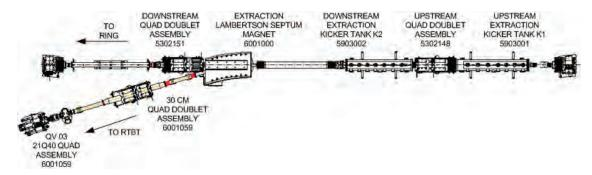
Figure 5.4. Extraction system magnets.
