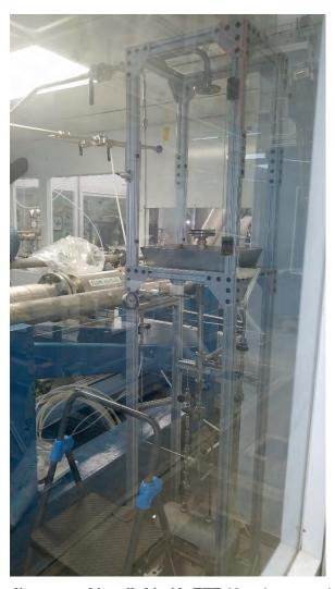
Figure 8.33. Filter media test stand installed inside TTF. Note the test section has been removed.
