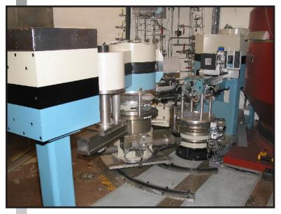
provide HB-1A with an exceptionally clean beam nearly free of higherorder contamination neutrons:  $I_{\chi 2} \approx 10^{-4} \times$ I<sub>2</sub>. This instrument has one of the most intense monochromatic neutron beams at the HFIR, as well as a very low background. Typical energy resolution is 1 meV (full-width half maximum at the elastic line), but this value can be reduced to 0.5 meV with the Be analyzer. Because of the combination of high
