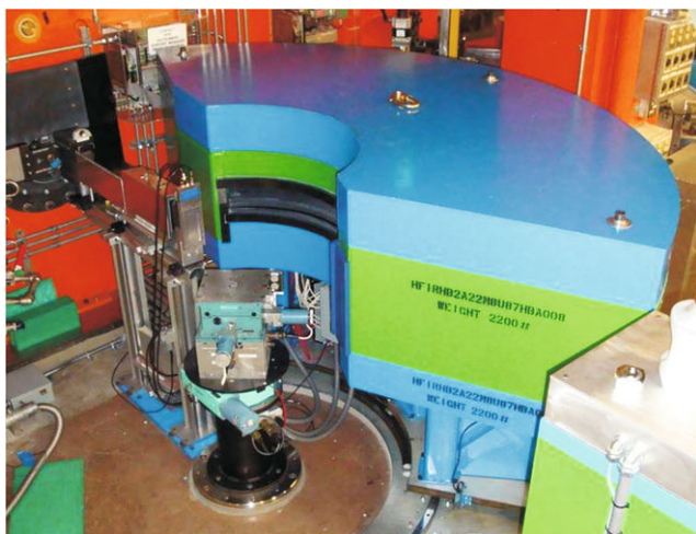
Fig. 1 The HB-2A high-resolution neutron powder diffractometer located at the High Flux Isotope Reactor, at Oak Ridge National Laboratory. The distance from the sample to the detectors is 1 m
