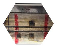
Advanced materials: US Navy researchers used HFIR neutrons to non-destructively evaluate the real-time effects of welding copper-nickel alloys commonly used in submarines and other naval vessels. The results could help limit or prevent solid-state cracking, which increases the likelihood of corrosion and reduces the life of the metals.
