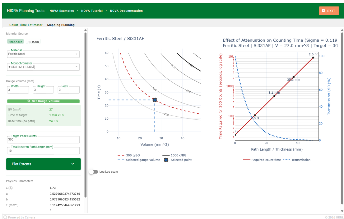
Figure 5. After clicking Set Gauge Volume, the count-time map shows a crosshair at the selected gauge volume with the required exposure time.
