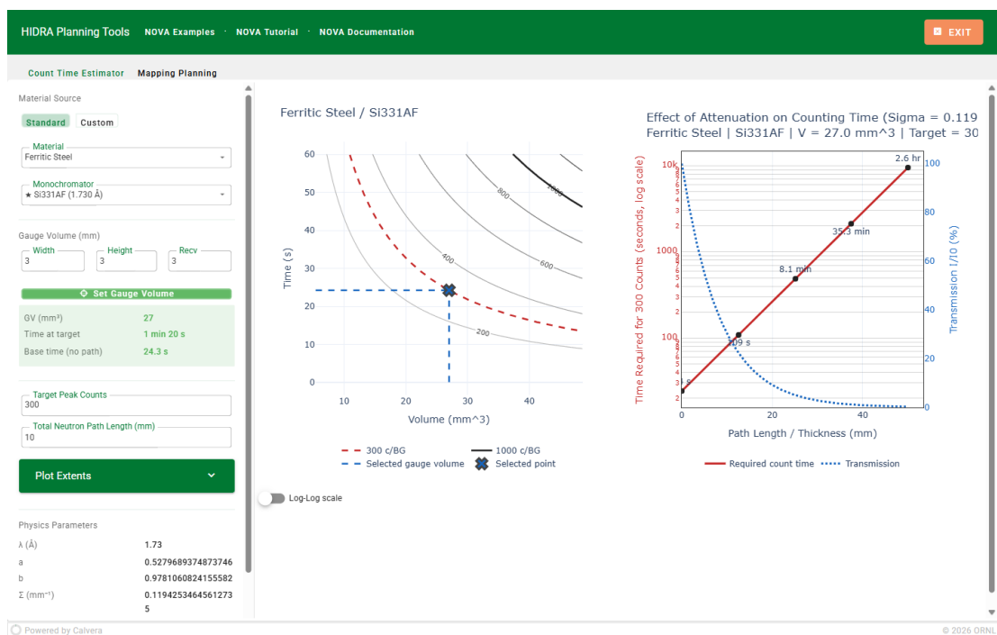
Figure 7. The Attenuation Count Time curve for Ferritic Steel / Si331AF. Required time grows exponentially with sample depth.
