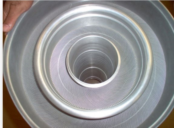
Figure 7: Top View of a HFIR Fuel Bundle
