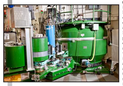
monochromator, the instrument is the ideal location for performing experiments at highenergy transfers (up to about 100 meV). The HB-3 monchromator provides three crystal choices (PG 002, Be 002, and Si 111) with variable vertical focus. This focus is calibrated to maintain a 2.54 cm beam height at the sample position, thus optimizing incident neutron flux as the incident energy varies. Of the three monochromators,
