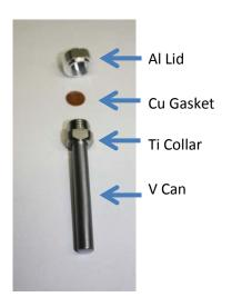
3. If present, remove film from Cu gasket to expose the mirrored surface. This may not be necessary as some gaskets have no film and are polished on both sides.
