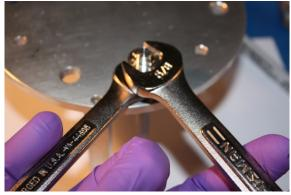
d. The wrenches should be held approximately 30-90 degrees apart so that the top wrench is to the right (CCW) of the bottom wrench.
