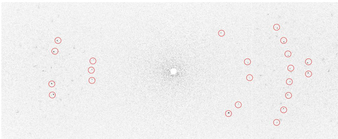
Figure (Top): Subtraction of a diffraction pattern collected at 20K from a diffraction pattern collected at 4K. Red circles highlight the magnetic super lattice peaks.
