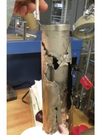
FIG. 3. Niobium embrittled by water at elevated temperature.
