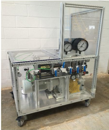
Gas Loading compressor
