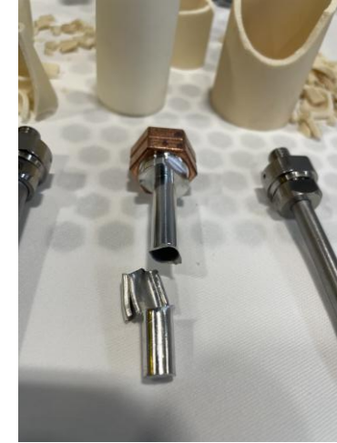
FIG. 3. Niobium embrittled by water at elevated temperature.
