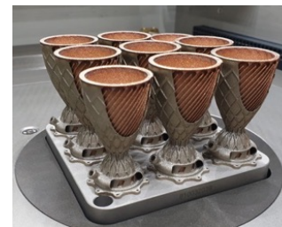
Multimaterial combustion chamber (LPBF)
