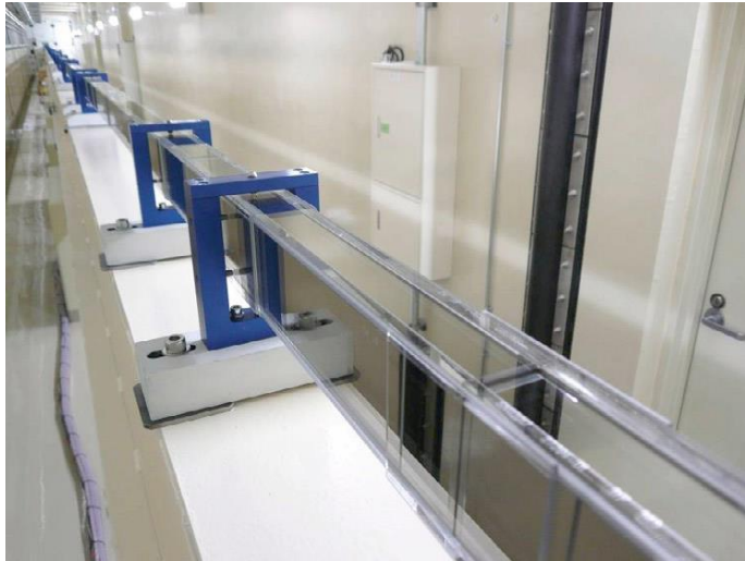
80m Guide for HRPD at J-PARC Fabricated by Swiss Neutronics
