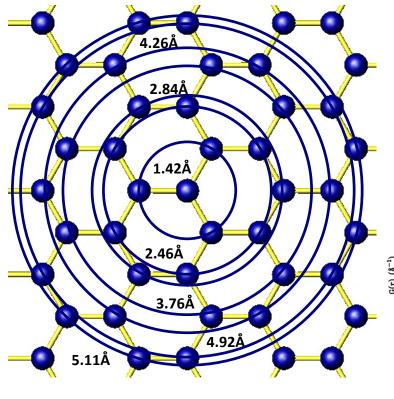
The Pair Distribution Function (PDF) gives the probability of finding an atom at a distance "r" from a given atom.
