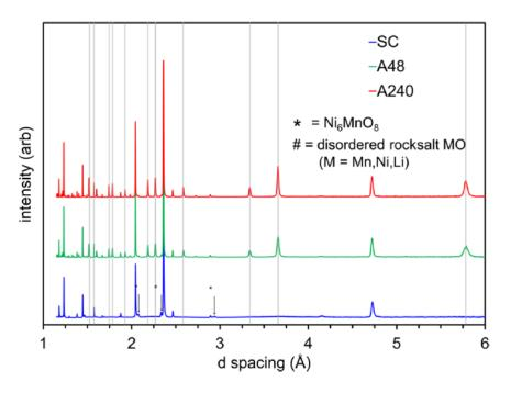
Cation ordering examined at the POWGEN Beamline, SNS: large nuclear scattering length contrast between nickel (*b* = 10.3 fm) and manganese (*b* = -3.73 fm)
