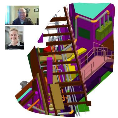
CAD model of gas cabinets and exhaust line
