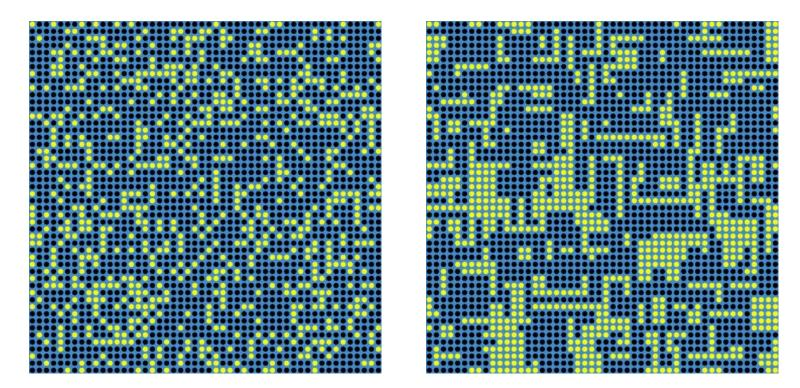
Cross section of 50x50x50 unit cell model crystal consisting of 70% blue atoms and 30% vacancies.
