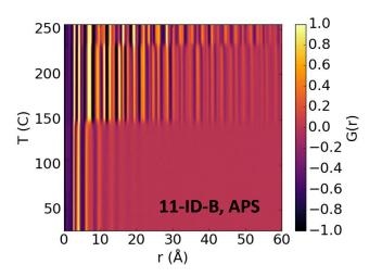
Data collected for 1  $\mu$ m films deposited **on kapton**, thermally annealed in situ under flowing He to 155°C and measured at ~60 keV in transmission K. Page, J. K. Baldwin, Th. Proffen, unpublished.
