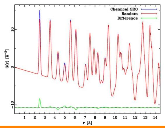
The PDF is the Sine-Fourier transform of the total scattering (Bragg and diffuse) diffraction pattern
