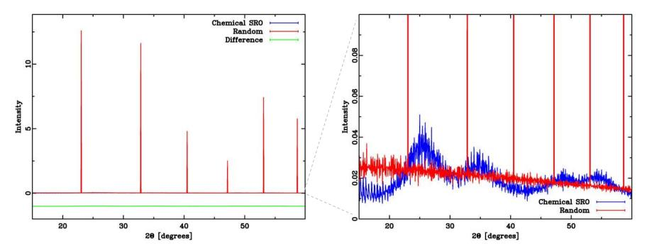
Bragg scattering: Information about the *average* structure, *e.g.* average positions, displacement parameters and occupancies
