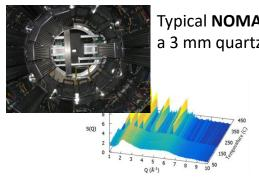
Typical **NOMAD** data can be collected for **30 - 100 mg** of sample in a 3 mm quartz capillary in ~**1 hour**
