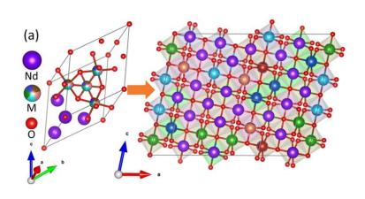
Primitive unit cell and Special Quasirandom Structures (SQS) supercell
