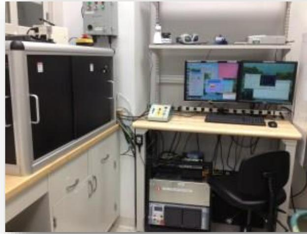
Gasket laser drilling system at GSECARS
