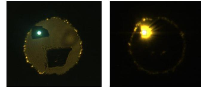
X-ray and lasers are aligned.
