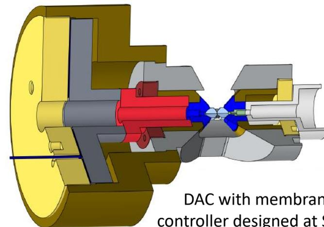
DAC with membrane controller designed at SNAP
