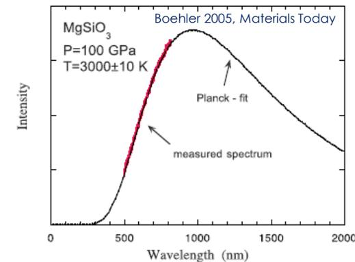
Thermal emission is measured.
