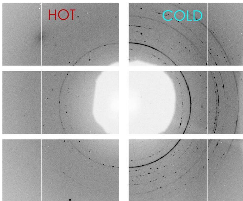
When a phase melts, peaks disappear, and diffuse scattering appears due to the liquid phase
