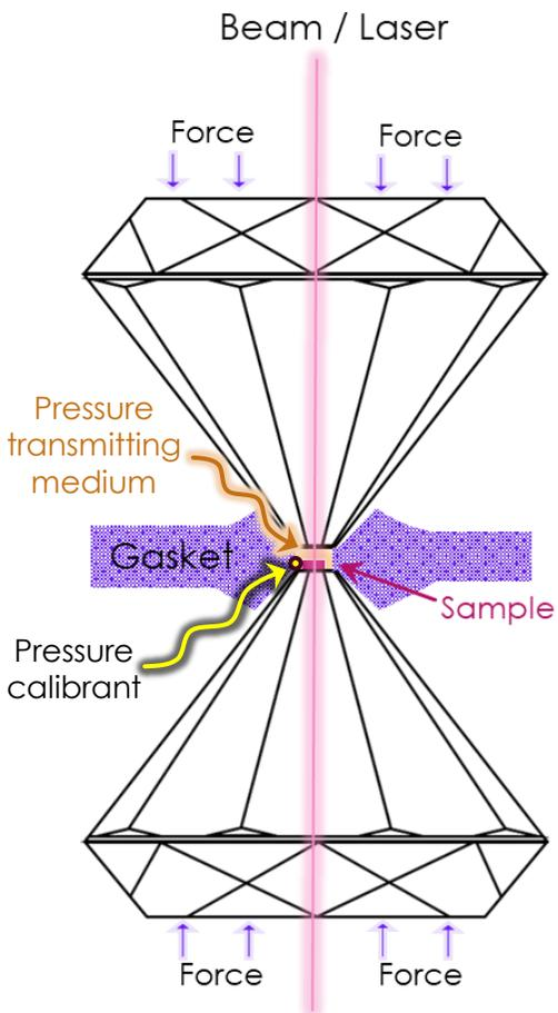
DAC is the most popular high-pressure device for X-ray experiments, because diamond has :
