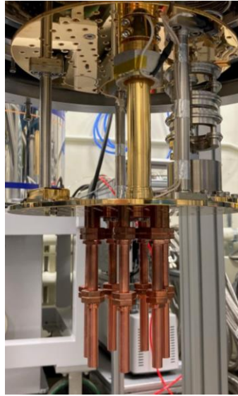
POWDER: Dry dilution fridge + 14 sample changer (base temp ~ 10 mK)
