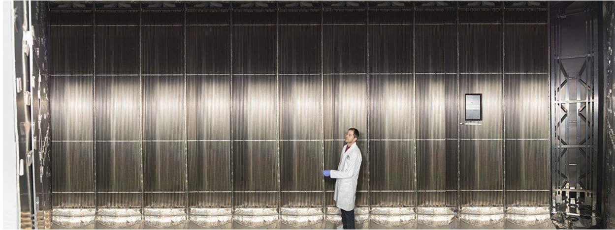
Detector Array at LET Spectrometer TS2@ISIS
