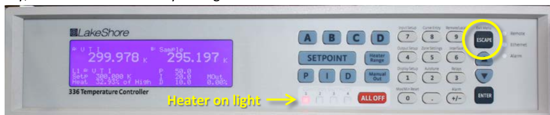
Figure 3. Lakeshore 336 temperature controller, showing the Escape button.
