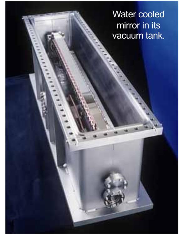
Most mirrors are made from silicon coated with one or multiple stripes of high-Z material after polishing.
