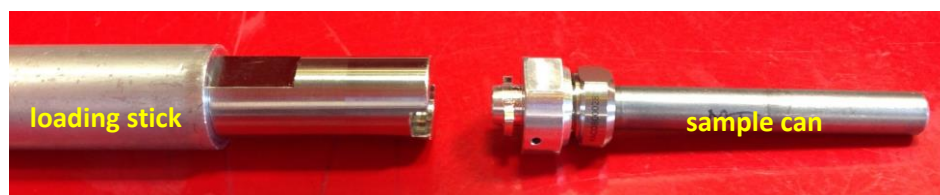
Figure 4. Sample loading stick, showing alignment with sample can lid.
