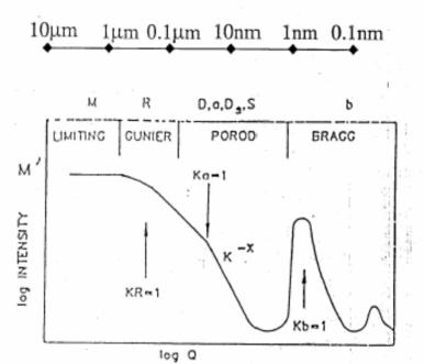
SANS is a structural technique that probes a wide array of length scales
