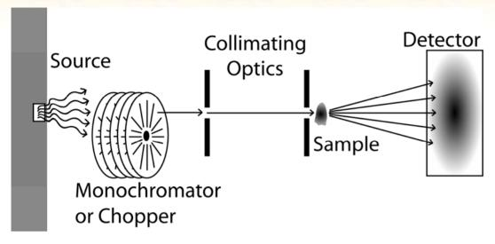
**Source:** A spallation source or a reactor
