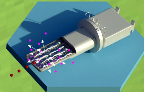
Once the protons leave the ring, they smash into a liquid mercury target, and "spallate" or create 20 to 30 neutrons for each interaction.
