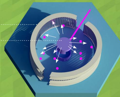
But here's the really cool part: The impact of neutrons on a sample material causes them to scatter at different angles—try to picture pool balls colliding—as the neutrons interact with atoms or magnetic fields in the sample materials.
