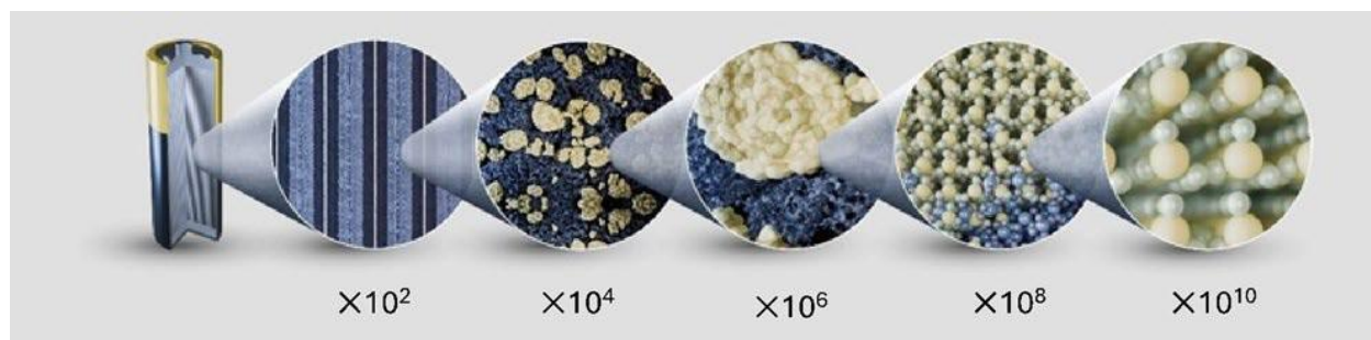
Figure 14. Multiscale structure of a battery cell. An illustration of the different length scales that are important to the function of a battery cell. Image courtesy of Phoenix Pleasant/ORNL.
