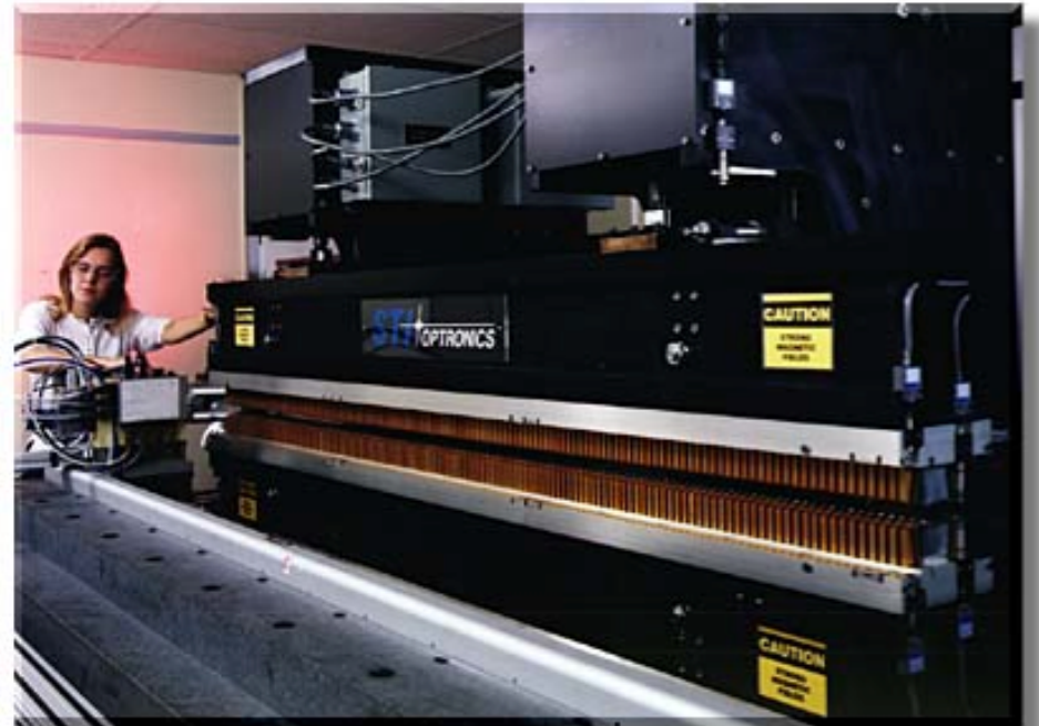
APS 2.4 m long Undulator A ( \lambda_{ID} = 3.3 \text{ cm} ) Permanent magnets
