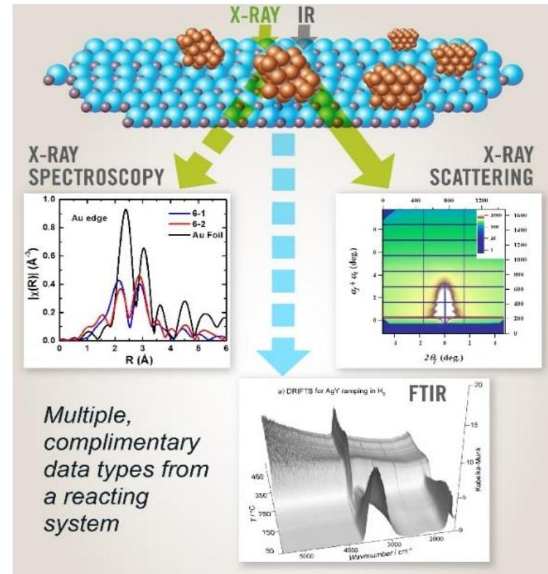
X-ray scattering and spectroscopy combined with FTIR and Raman to study in situ catalysis on a flat surface.
