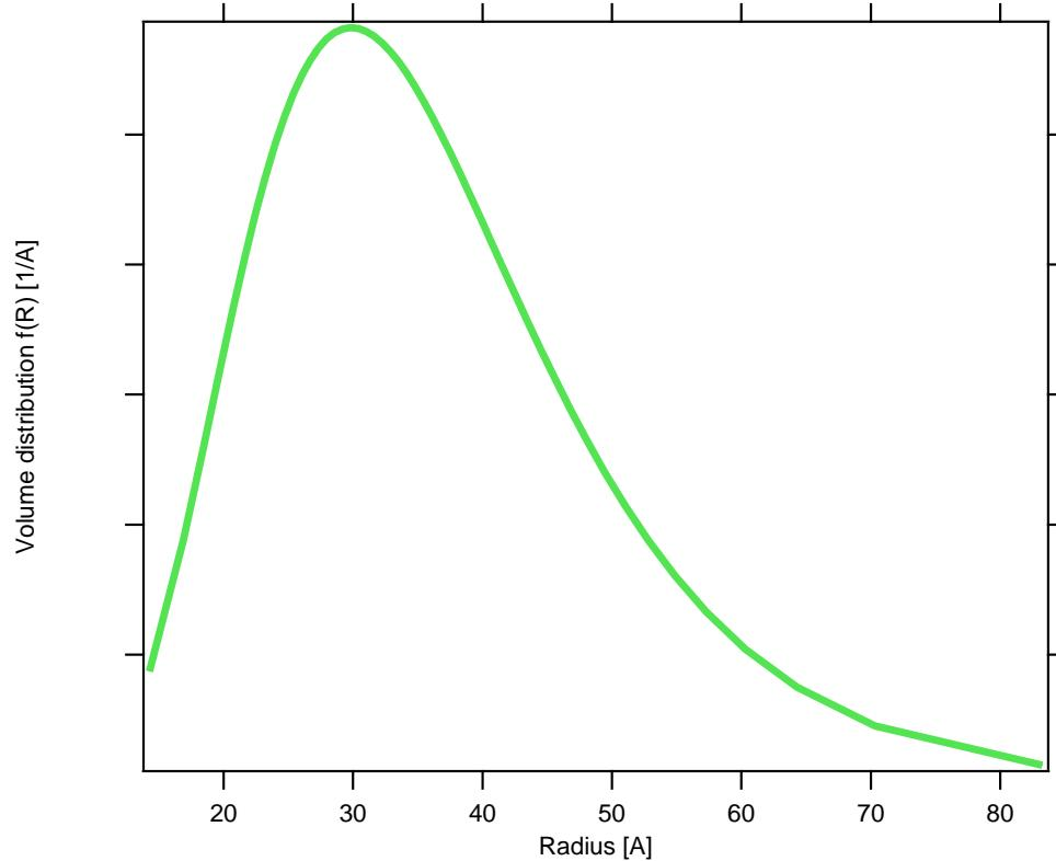
The fitting shows that the average particle size is 6.7 nm, consistent with BJH Model data 7.1 nm.
