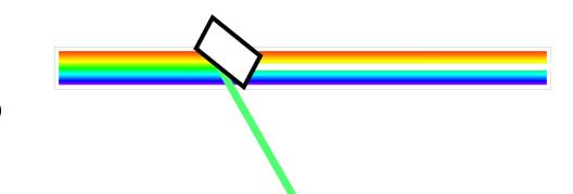
Can re-use the transmitted beam for other wavelengths!
