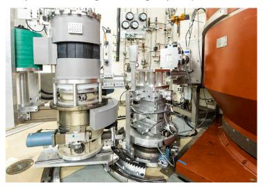
signals. VERITAS is also an exceptional instrument for diffraction studies under extreme conditions requiring variable temperatures (T), magnetic fields (H), high pressures (P), and electric fields (E).
